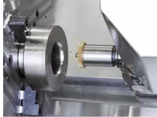
Shaping of external gear teeth (Flanx-Spline)
