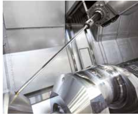
▼ Deep hole drilling
